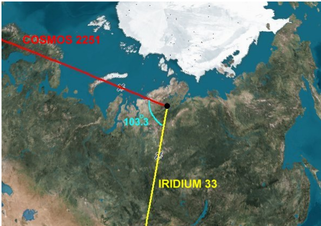
Figure 3: The collision angle of Iridium 33 and Cosmos 2251 as viewed from directly above the collision point, denoted by the black dot. Earth and orbit imagery by Analytical Graphics Inc.
