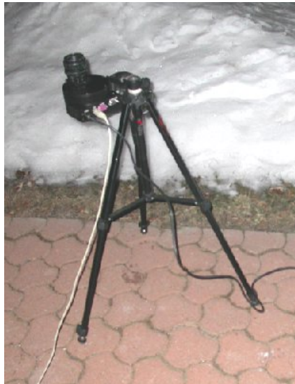
Figure 7: My ST-9XE CCD camera mounted on a simple tripod. The CCD camera was fitted with a 50mm lens and pointed at my local zenith with the aid of a simple bubble level. It caught LEO satellites as it continuously took images of the zenith with an 11.2 by 11.2 degree field of view.
