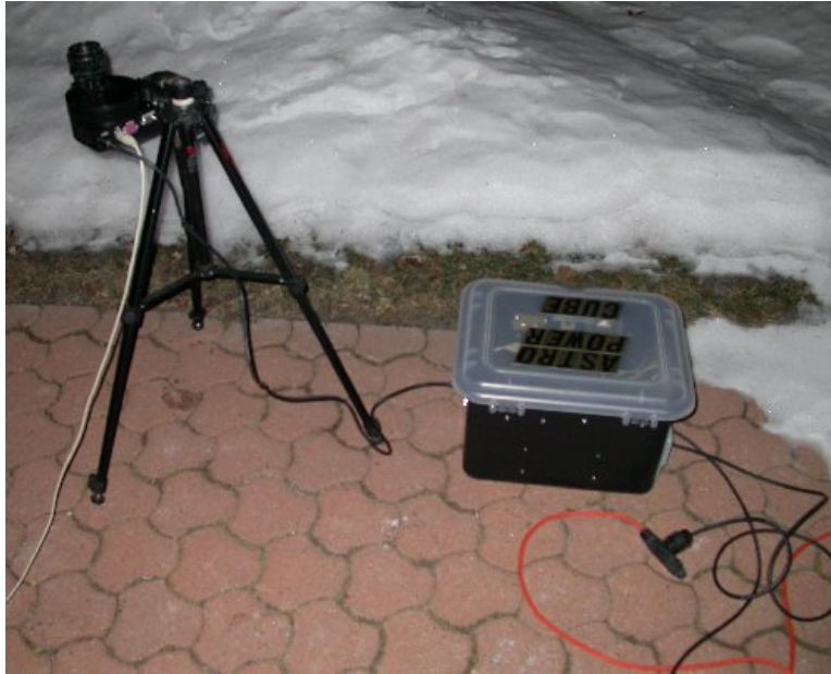
Figure 4: My ST-9XE CCD camera on a simple tripod connected to the “Astro Power Cube” during testing. The camera obtained about 1000 images of my local zenith without incident. The images were sent to my laptop located indoors.
