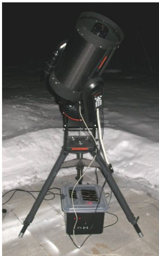
Figure 5: The “Astro Power Cube” in action. Both the telescope and the CCD camera are connected to the device with low-temperature cables. If the cables should crack or break they can be replaced without having to touch any of the power supplies themselves. The dew heater is not connected in this image. If you look closely, you can see the telescope and CCD camera power indicator LEDs lit up on the cube!
