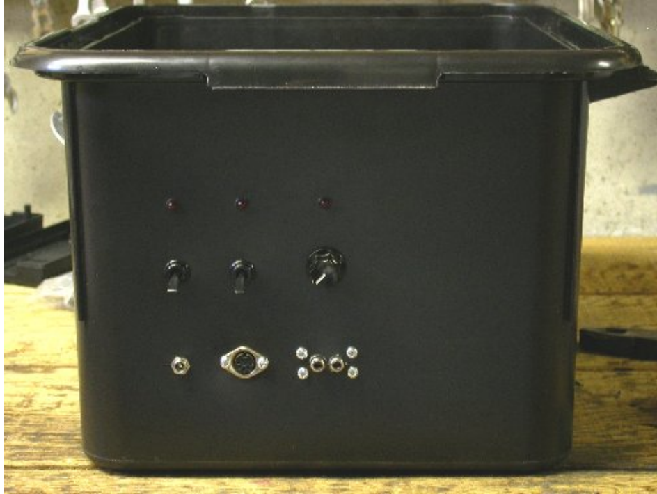
Figure 3: The “power supply” side of the “Astro Power Cube”. Power outputs for the telescope, CCD camera and the dew heater are shown here. I left extra space for any additional accessories. The dew heater’s temperature control variable resistor was removed from the original box and placed on the cube’s side wall.
