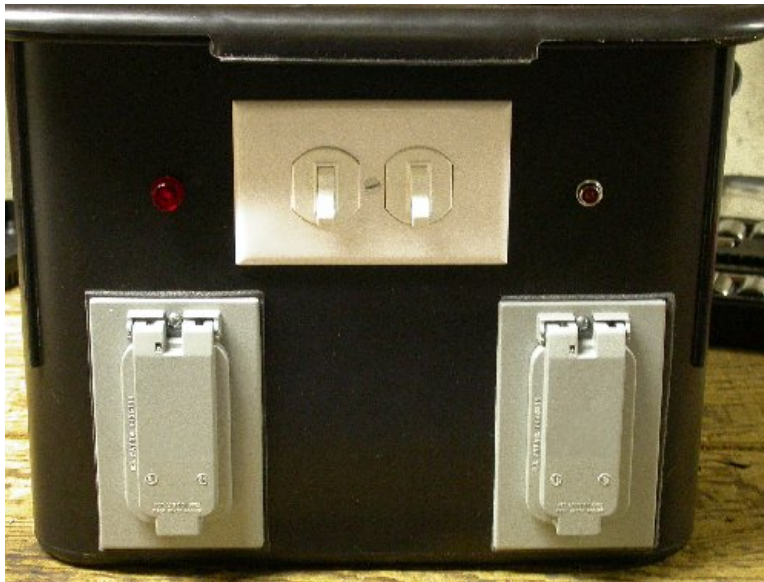
Figure 2: The “high voltage” side of the “Astro Power Cube”. It features two power outlets per power source. The left-hand outlets would be for the 120VAC main power (for home use), and the right-hand outlet would be used for the 12V inverted power (for star party use). The switches on the top are the main power switches for the 120VAC main (left), and the 12VDC (right). The indicator lamps are there to indicate when the main power and/or the 12VDC power are active. Note the protective covers on the two power outlet assemblies.
