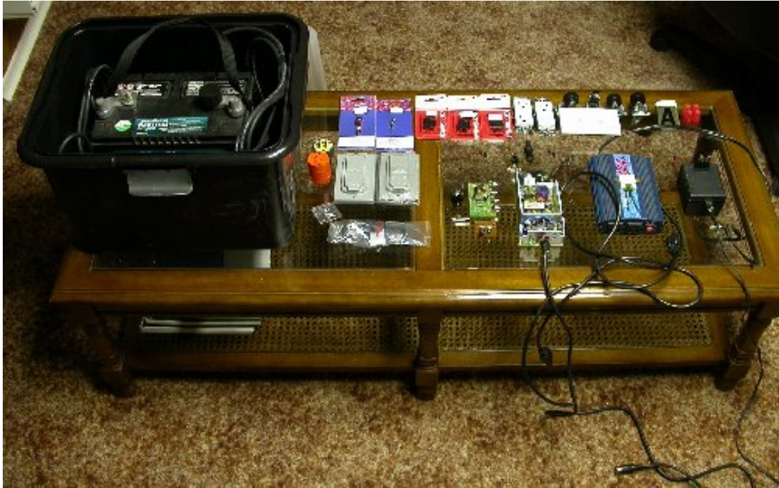
Figure 1: The component parts to the “Astro Power Cube”. The power supplies to the telescope and CCD camera, as well as the inverter and dew heater assemblies would be installed. The letter file box is shown at the left, along with the 12V deep cycle battery that would power the dew heater and the inverter.
